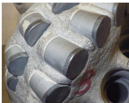
Figure 5. 6 1/8 in. Horizontal Series - SH513DE dull bit with HD Cutters.
