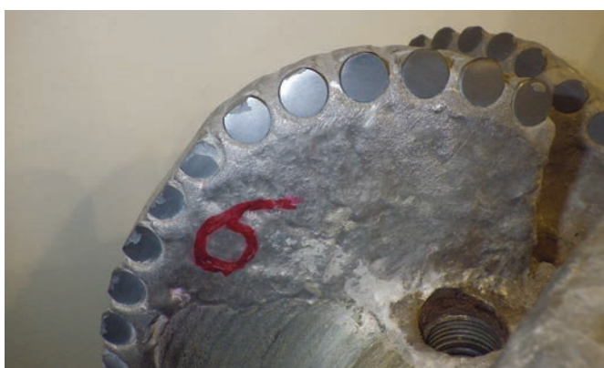
Figure 2. Dull condition of first SHEAR BITS 16 in. SV613 run with HD Cutters™.
