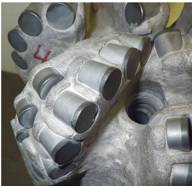
Figure 6. 6 1/4 in. Horizontal Series - SH613DE dull bit with HD Cutters.
