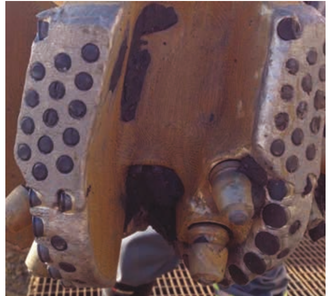
Figure 7. Dull condition of a 12 ¼ in. Pexus hybrid bit after completing a challenging S curve interval.
