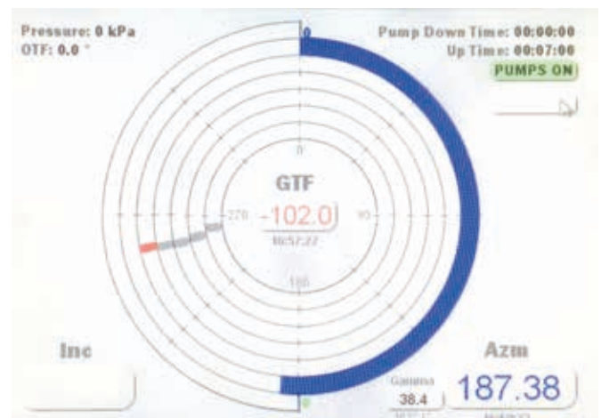
Figure 8. Photo of toolface plot taken during a slide in the 6 ¼ in. SHP613D run.
